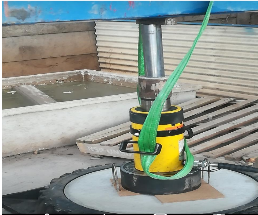
Figure 1: Testing of Prototype Reinforced Concrete Drop-in Cover Type 2A. Note the Standard cast-iron type 2A frame.
